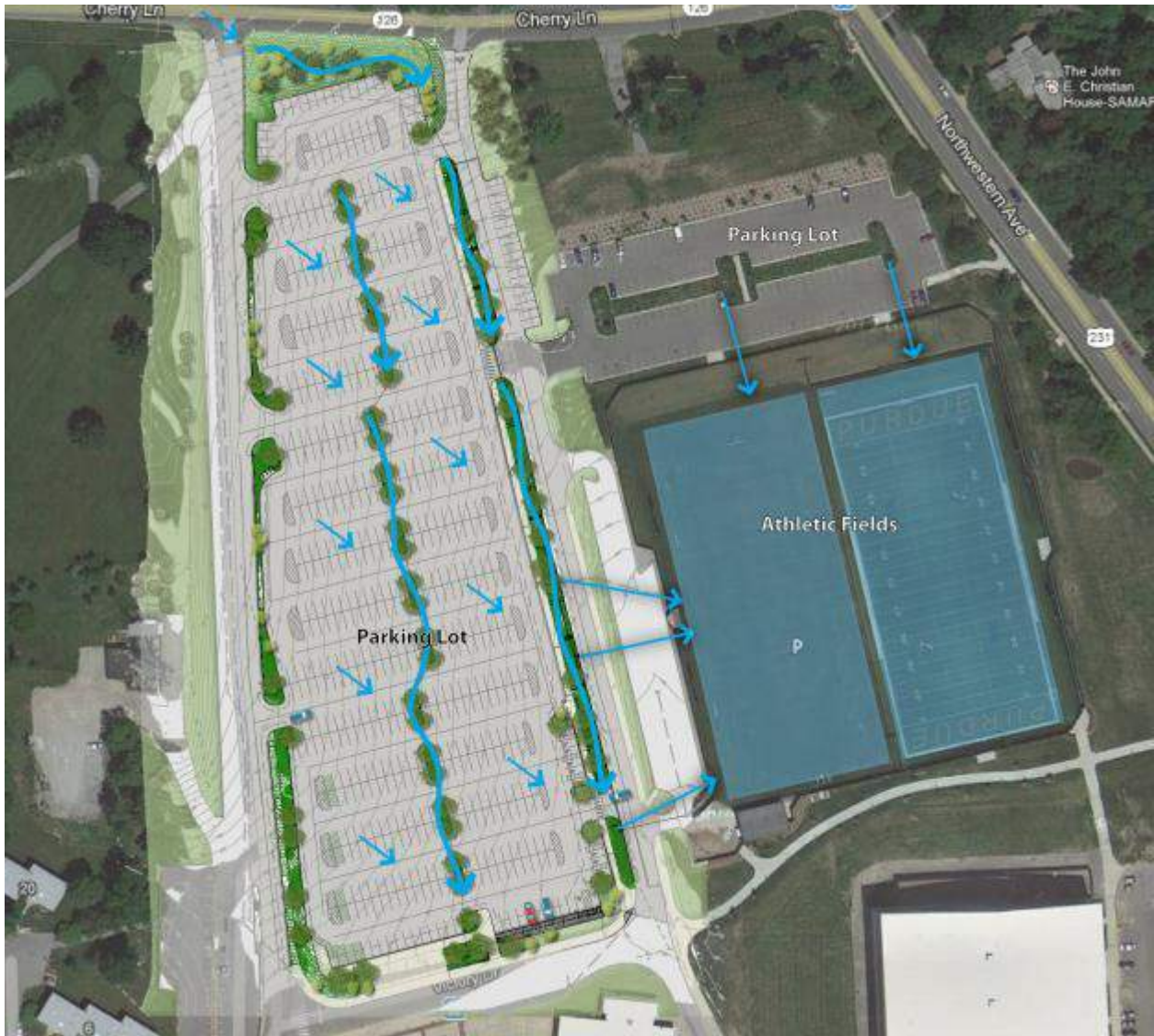
Figure 5.3.2-7. This diagram of the athletic fields at Purdue indicates how runoff from streets and parking areas is directed through bioretention areas and vegetated swales before being directed to the infiltration bed. Overflow from the vegetated systems is piped into the bed in this “treatment train” approach.
