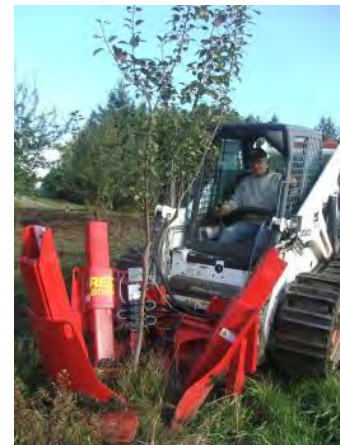
Figure 5.2.4.2-10. Small tree salvage.
