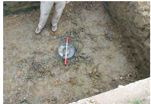
Figure C-2. Double-ring infiltrometer test.
