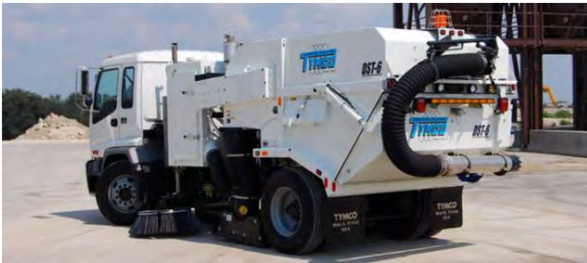
Figure 5.5.1-1. This regenerative air street sweeping unit removes both large debris and fine particulates ( http://www.tymco.com/sweepers/model-dst-6/index.htm , accessed August 2012).
