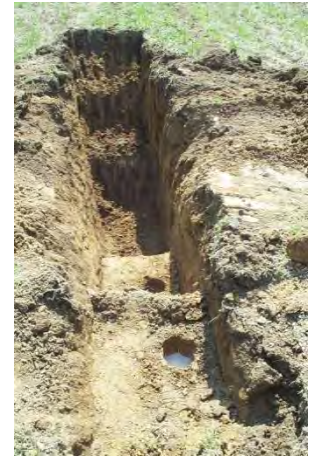
Figure C-1. Soil test pit.
