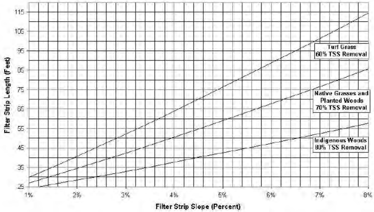
Figure 5.3.6-3.c. Graph may be used to estimate filter strip width based on soils, slope, and vegetation. Adapted from New Jersey Stormwater Management Practices Manual, Chapter 9, 2004.
