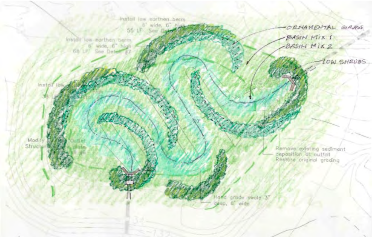
Figure 5.3.13 -3. Concept rendering showing how berms can be used to increase the flow path through a naturalized basin.
